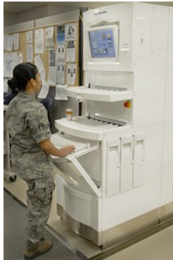
Airman 1st Class Roma Terry, a pharmacy technician with the 18th Medical Support Squadron, begins running a check on the new pharmacy robot. The PharmASSIST ROBOTx has established quality checkpoints throughout the pharmacy by employing bar code scanning, digital images of medications and original paper prescriptions, and protocols at every stage of the prescription filling process. (U.S. Air Force photo/ Airman 1st Class Tara A. Williamson)
