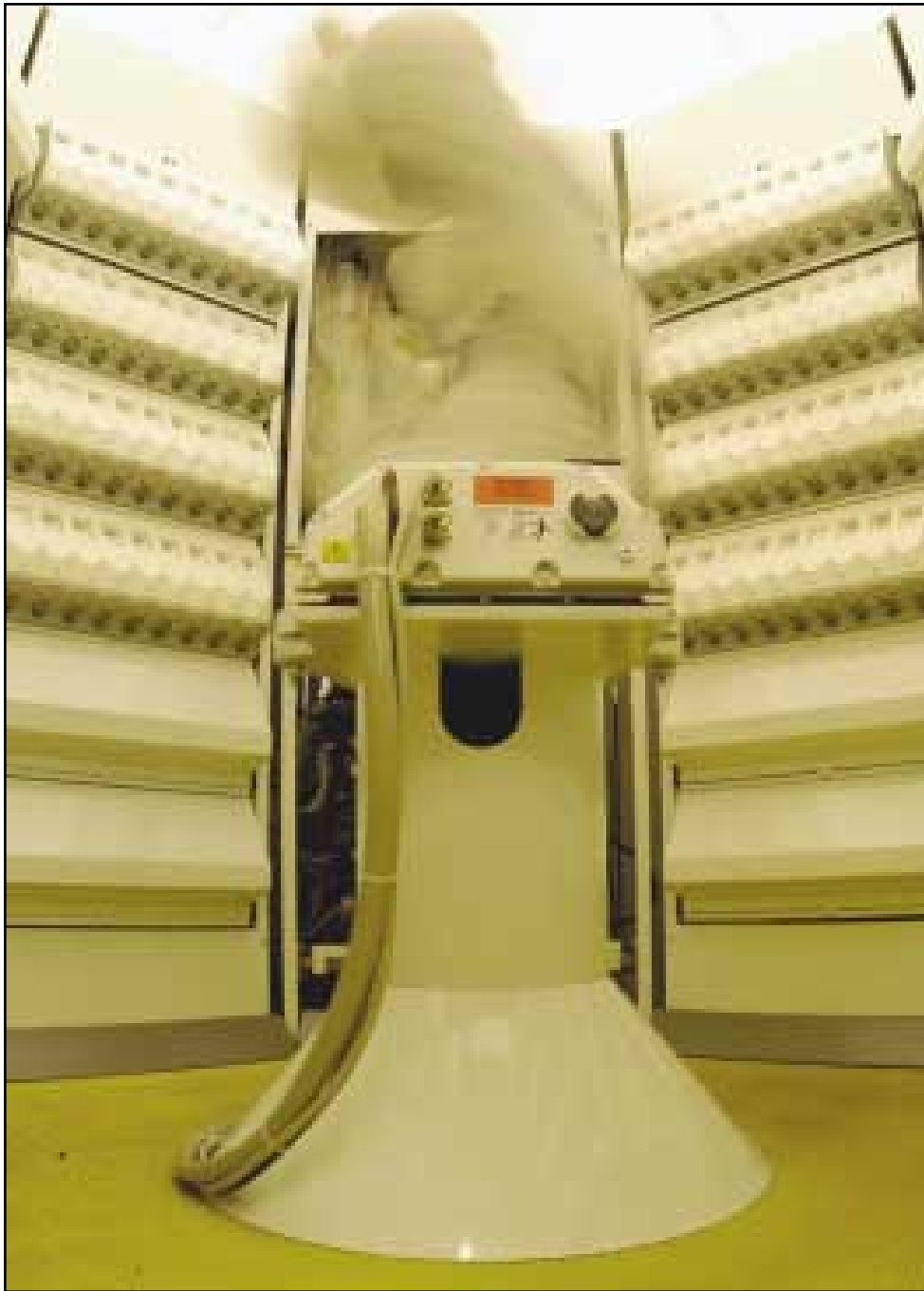
Each of the two robotic arms need only two hours to fill as many prescriptions as a busy pharmacist can complete in one day.
